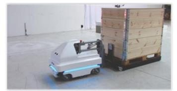
Automated Pallet Fork. The mobile robot can locate the pallet fork and transport it to it's destination autonomously. In this way the employees only have to load and unload the pallet from the pallet fork and they save valuable time, because they do not need to do the transportation themselves.
