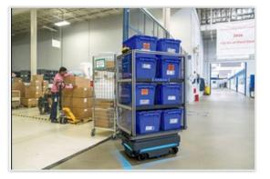
**Shelf Units** the shelf units are often used to transport semi-finished or finished goods between productions, between production and warehouse and/or in warehouse logistics. Shelf modules are often used in semi-automated installations, where an employee fills up the robot with the goods and send it on its way with just one click on a button.
